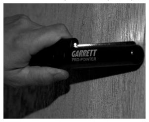
condition of the *PRO-POINTER* is monitored continually. When the battery becomes low, the detector will sound an alternating dual-tone alarm. This sound indicates that the detector's 9V battery should be replaced as soon as possible.
