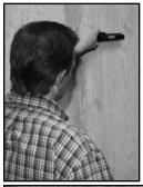
(Left) For wall scanning with a PRO-POINTER, use the side-scan technique to quickly cover large areas.
