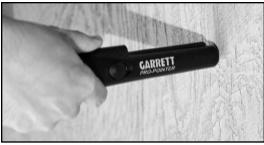
**Pinpointing Large Objects:** When locating large metal objects—whether in the ground or in a wall—you can improve the pinpointing capability by "detuning" the *PRO-POINTER* in order to narrow the detection field, as follows.
