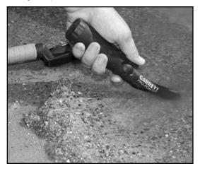
**Wall Searches:** The *PRO-POINTER*'s static mode makes it an excellent utility locator to find metal studs and pipes in walls or nails in the drywall. Use the side-scan technique to quickly cover large areas and use the pinpointing tip to precisely locate the target.
