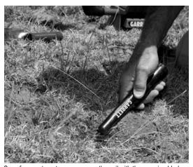
Scan for your target as you scrape the soil with the scraping blade.
