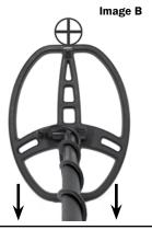
Once the target signal drops off (both audibly and on the LCD meter), shallow targets should be located immediately in front of the searchcoil's tip (see Image B). Deep targets will be under or just inside your searchcoil's tip. This is because the conical shape of the searchcoil's detection field begins bending in slightly as the depth increases (see Image C).
