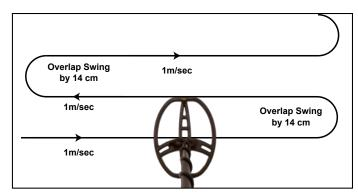
In order to fully search an area, overlap the swings of your searchcoil by half the length of the coil (about 14 cm). Sweep the searchcoil in a straight line or with a slight arc at a sweep speed of about 1m/sec.
