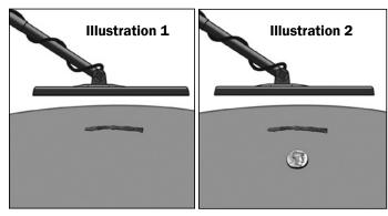
Iron targets, such as the nail shown above, can sometimes mask a good target. If too much iron discrimination is applied, the good target can be missed. Read page 23 to learn how to apply the proper amount of iron discrimination to eliminate the nail shown in Illustration 1 and still detect the good target shown in Illustration 2.
