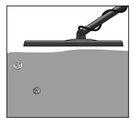
You can reverse this pinpointing technique to pinpoint off the DD coil's tail; in this case, push the coil away from you. The audio and LCD meter will place the target just off the searchcoil's tail.
