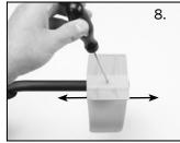
8. Adjust the arm cuff by removing the screw on the bottom and moving it to the other hole.
